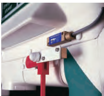
Proximity switch detail
